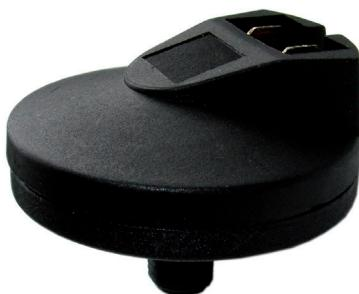
The maintenance switch (MS 55 - MS 65t), made of plastic, monitors the degree of contamination of air filters. When the switching point is reached, the switch sends an electrical signal, indicating that filter maintenance is necessary. This also prevents potential damage to the compressors, which could be caused by irregular service intervals.
