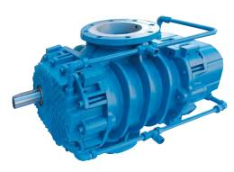
The blower is equipped with two cooling coils that keep the oil temperature below 100°C in all operating conditions. This version is recommended when the gas discharge temperature exceeds 140°C.
