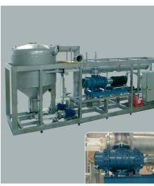
Engineering: treatment of oil emulsions and cleaning liquids by means of thermocompression concentration system.
