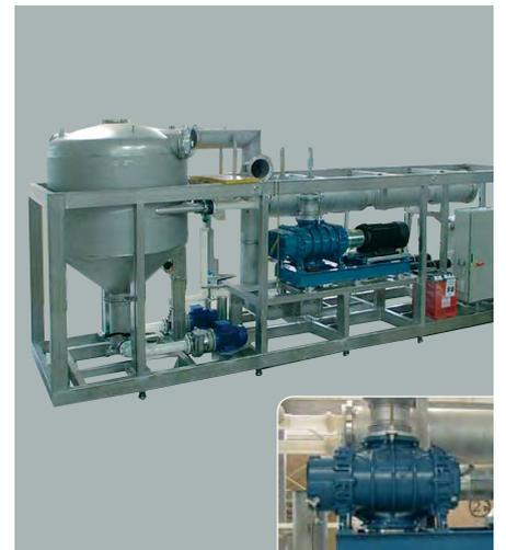
• Engineering: treatment of oil emulsions and cleaning liquids by means of thermocompression concentration system.
